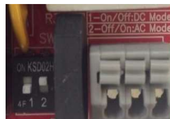
For DC Mode, #1 switch turn "OFF" and #2 switch turn "ON"
